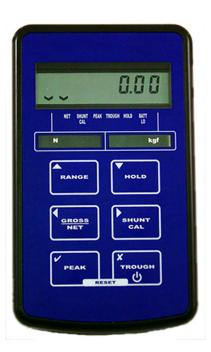
The <u>TR150 handheld display</u> is a completely portable high precision instrument designed to work with all types load cells and strain gauge based transducers. The 7-digit LCD display makes it suitable for any monitoring application from general industrial up to high accuracy reference standards.
